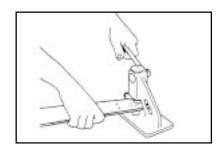
Figure 24. Punching out Nose Sprocket Rivets
