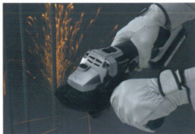
Reinforcing bar cutting
