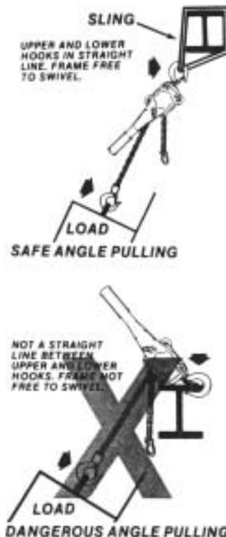
Figure 4 - Pulling at an Angle
