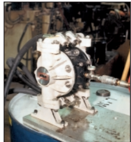
1/2" pump pulls cutting oil from a 55-gallon drum
