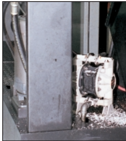
This 1/2" pump transfers cutting fluid through a filtering chamber
