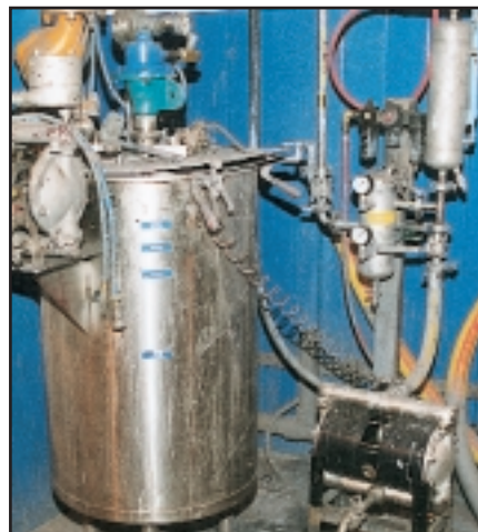
A 666101-244 (1" Stainless Steel) and 6661M1-2A4-C (3:1 Power Pump) are used in a mixing/recirculation process
