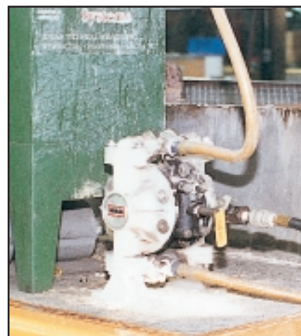
This 666053-322 (1/2" Polypropylene) is used on a parts wash rack
