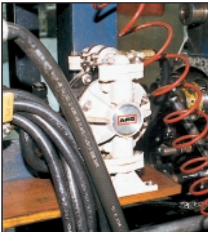
A remote-actuated 1/2" pump supplies oil on an "as-needed" basis
